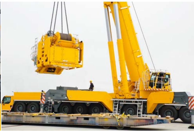
⑥ Self-assembly counterweight frame with drive assembly
