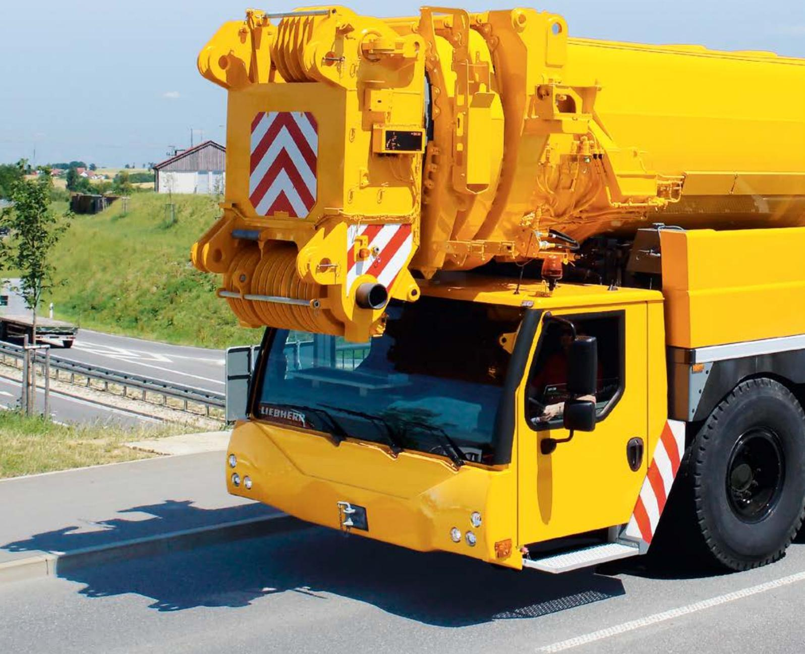
The LTM 1750-9.1 can carry the 52 m long telescopic boom, two folding outriggers and the main winch within the maximum axle load of 12 t. Considerable capacity increases are accomplished with the Y-telescopic boom suspension. Short set-up times, an extraordinary mobility as well as extensive comfort and safety appointments mark the mobile crane LTM 1750-9.1 from Liebherr.
