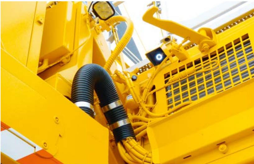
Camera monitoring of the slewing platform
