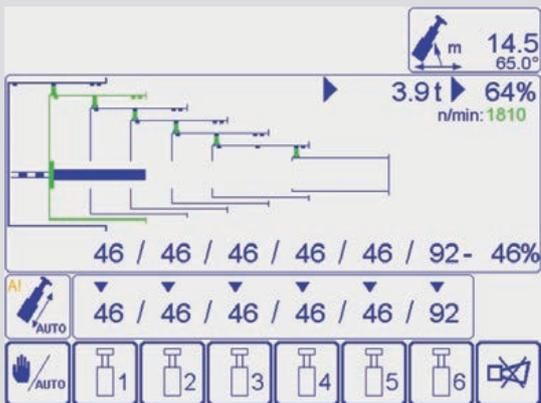
**The fully automatic telescoping system „TELEMATIK“**
